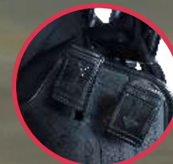
HYDROSTATIC TRANSMISSION WITH TWIN HST PEDAL
